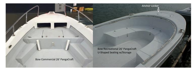
The difference is the commercial model has anchor locker. The Recreational has U-Shaped Seating with storage and anchor locker at the top of the bow.
